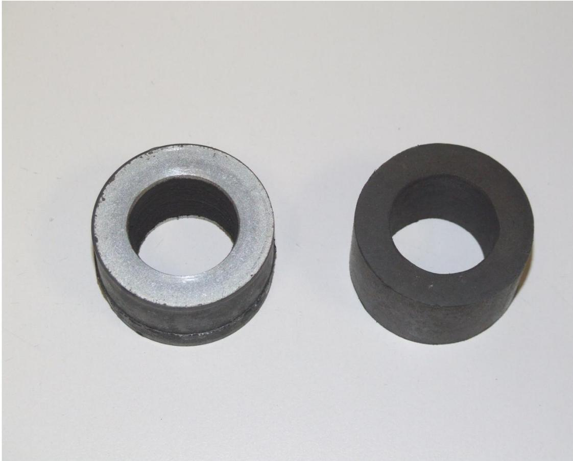
Fig. 1: Rubber damper with volcanized metallic discs ,old' rubber damper (to be replaced)
